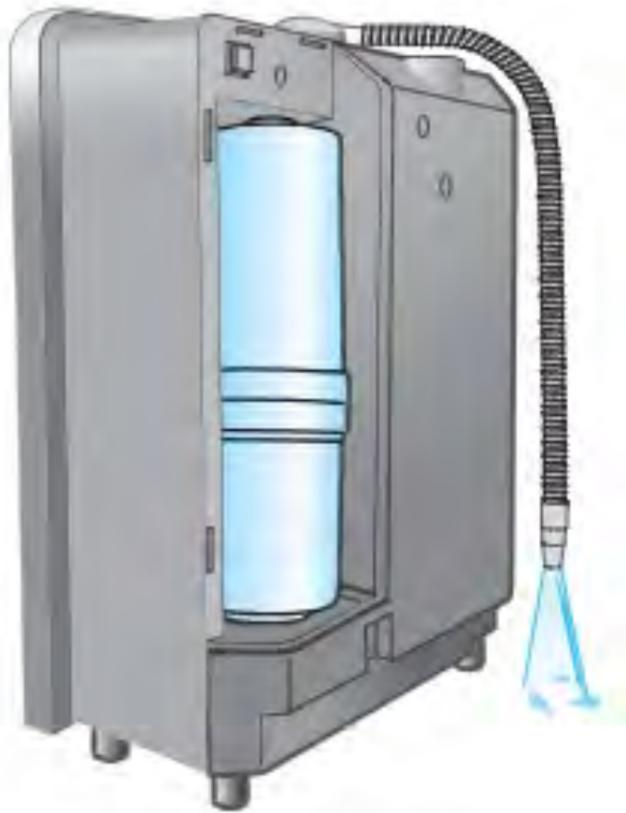
Now switch the main switch ON again, open the water supply with the turn dial and test the new filter to see if it is sealed for 2-3 minutes.
