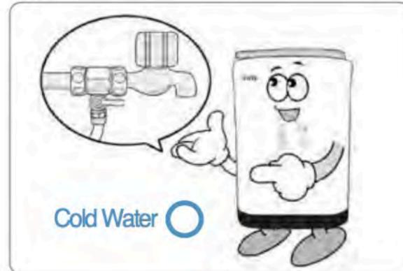
Connect the ionizer only to cold water supply. Damage resulting from connecting the ionizer to hot water supply is not covered by the warranty.
