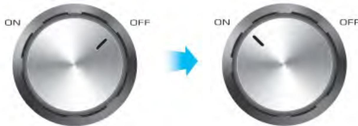
With the turn dial you regulate the water flow from 0 (OFF) to Maximum (ON). Once water flows, the display indicates the operating status and an announcement is made in English. Tip: How far you turn the dial has a direct influence on the ionising performance of your water ionizer. With a slower flow does contact time and therefore ionization of water increase.
