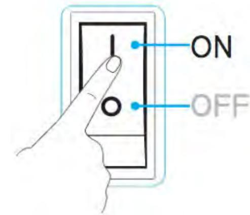
You will hear a signal tone and the display panel will light up for 2-3 seconds. When the main switch is on and the display panel is not illuminated the ionizer is in standby mode.
