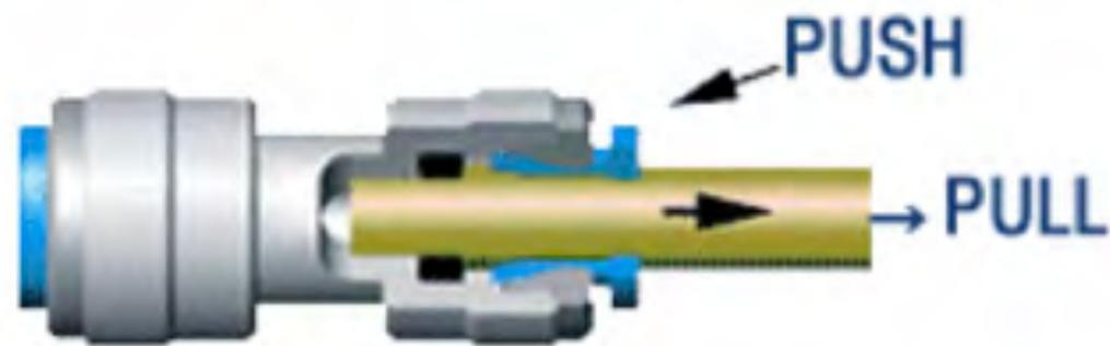
If you do not have long finger nails it can be difficult. A screwdriver or knife can help. Attention: The pipe can only be released if it is not under pressure. Please ensure that you have released the pressure by shutting off the flowing water supply at the T-piece or the faucet. Like this the pressure is released safely and the plug caps can be released in the above described manner. For safe transportation is the original packaging suitably the best, which should be kept if possible.
