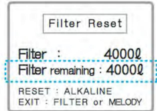
Press the FILTER button for 3 seconds until Filter RESET is displayed. Now press the ALKALINE button for 3 seconds until the remaining service life of the filter indicates 4000 L.
