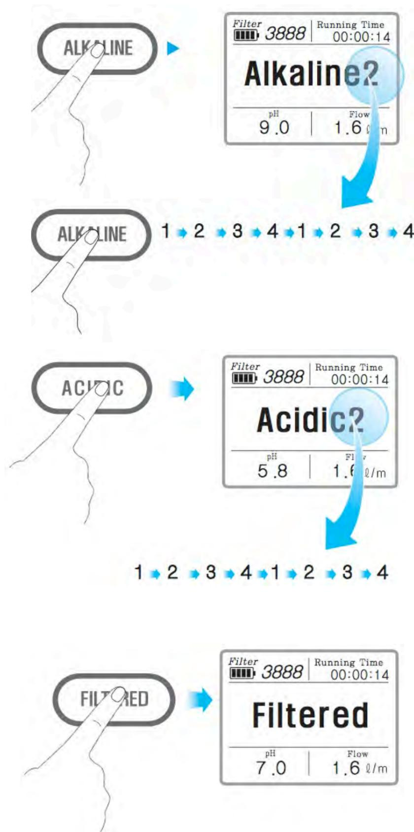
When alkaline water flows out of the Stainless Steel flex-hose, acidic activated water flows out of the outlet pipe into the sink. The reverse happens when you choose ACIDIC, which can also be set to 4 levels. You will always get the selected water type from the Stainless Steel flex-hose. Acidic water can be used to rinse fruit and vegetables, for skin care and to water the plants.
