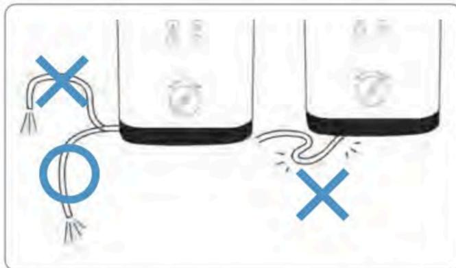
Acidic water tubing must not be raised higher than the base of the product.
