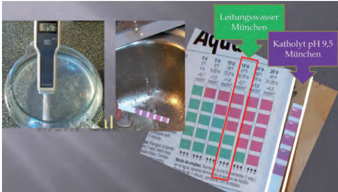
Above: Tap water Munich (green). Electrolyzed alkaline tap water Munich (purple). So the content of \text{CaCO}_3 increased from > 2,7 \text{ mmol/m}^3 to > 4,5 \text{ mmol/m}^3 .
