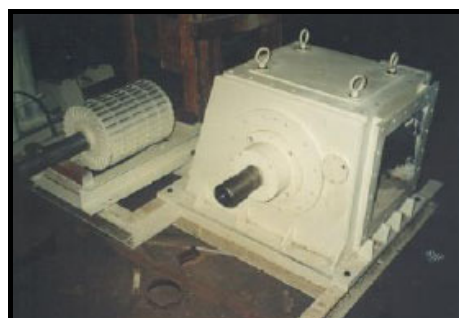
Figure 29: Cross Flow Turbine,
