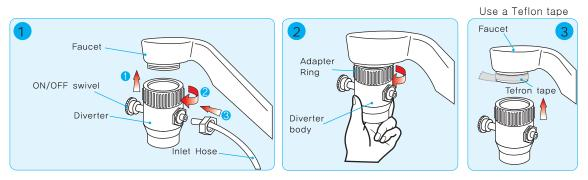
on the bottom of the ionizer labeled "TAP WATER INLET" . To attach the white hose, simply push it firmly into the opening on grey port. (If you need to remove it, press on the end of the fitting
