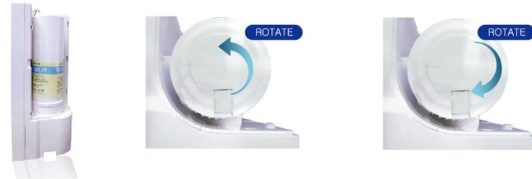
4. Rotate the first or second filter to the left to detach it from the equipment.
